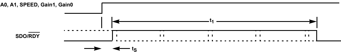
FIGURE 28. \overline{\text{SDO}}/\overline{\text{RDY}} DELAY AFTER MULTIPLEXER CHANGE
