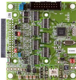
When connected to a DC9003A-C Evaluation/Development Mote, the **DC9006 Eterna interface card** provides a USB connection for both power and software access to the mote API UART port.
