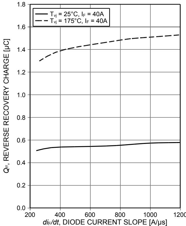
Figure 5. Typical reverse recovery charge as a function of diode current slope ( $V_R=400\text{V}$ )
