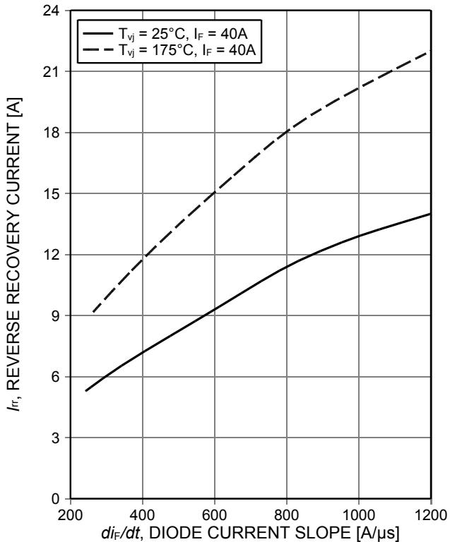
Figure 6. Typical reverse recovery current as a function of diode current slope ( $V_R=400\text{V}$ )
