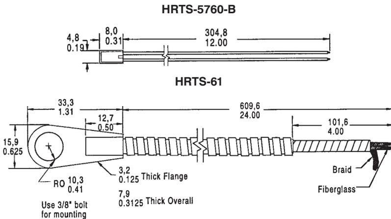
The HRTS is designed to measure surface temperatures from  $-200^{\circ}$  to  $+480^{\circ}$ C ( $-320^{\circ}$  to  $+900^{\circ}$ F) in printed circuit, temperature probe, or other applications.
