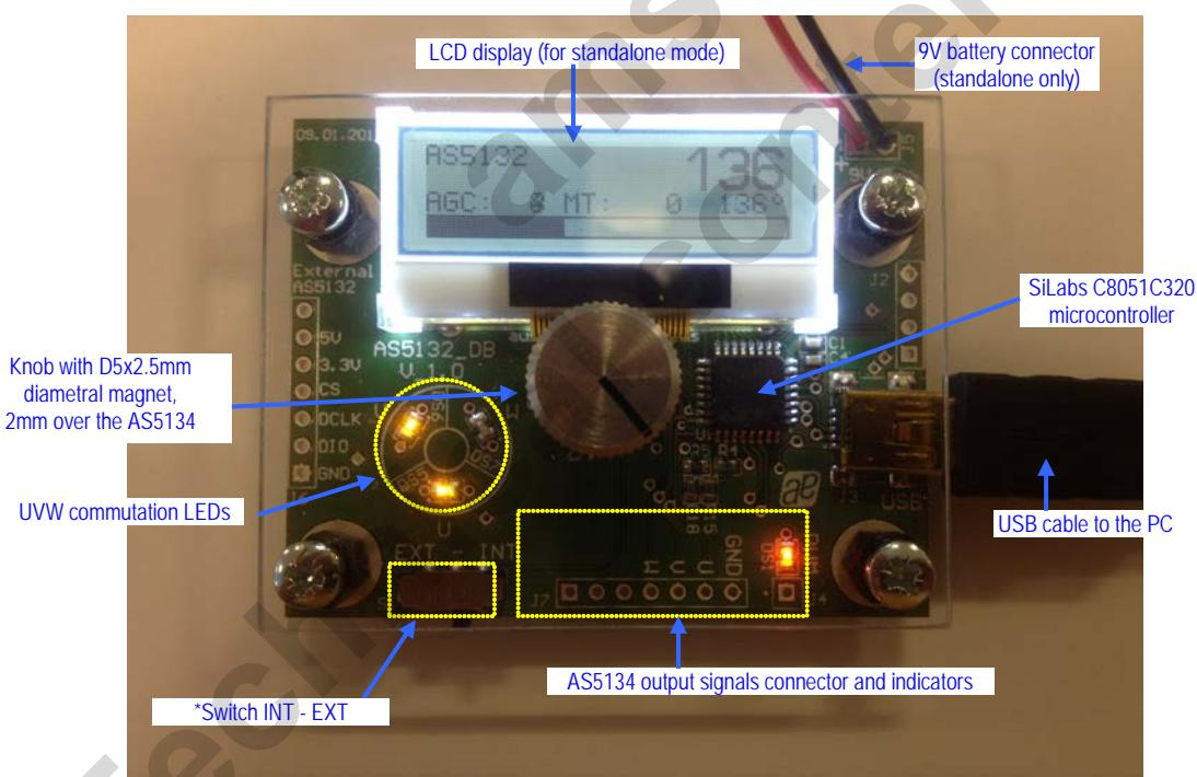
Figure 1: AS5132 Demoboard hardware with mounted magnet knob
