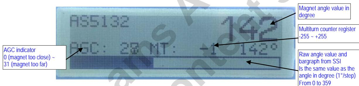
Figure 2: LCD display in standalone mode (9V battery or USB powered without GUI)
