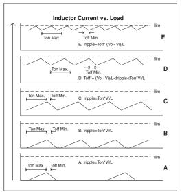
Figure 1. Inductor Current vs. Load
