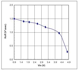
$\overline{K_{OFF}}$  vs.  $V_{IN}$ ,  $V_{OUT}$ =5.0V
