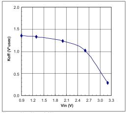
$\overline{K_{OFF} \text{ vs. } V_{IN}, V_{OUT}} = 3.3V$
