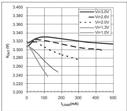
Line/Load Rejection vs. Load Current,  $V_{OUT} = 3.3V$
