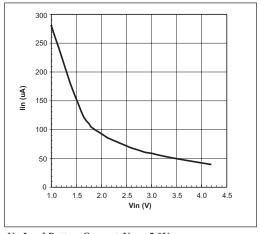
No Load Battery Current, V<sub>OUT</sub>=5.0V
