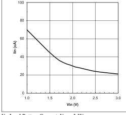
No Load Battery Current, V<sub>OUT</sub>=3.3V
