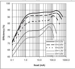
Efficiency vs. Load Current,  $V_{OUT}$ =3.3V
