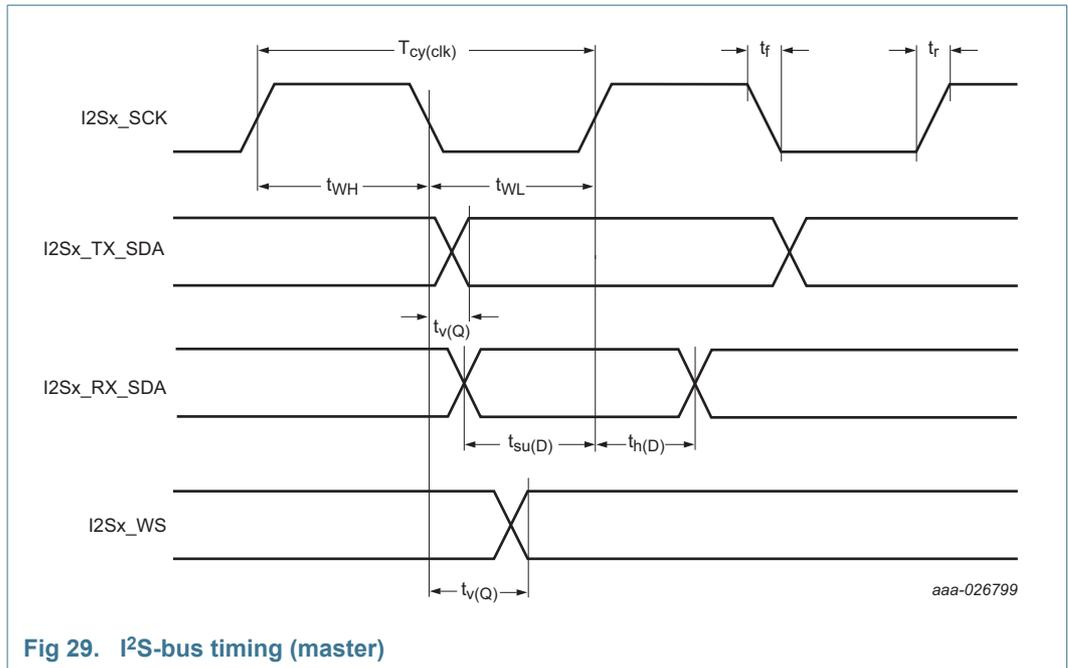
Fig 29. I<sup>2</sup>S-bus timing (master)
