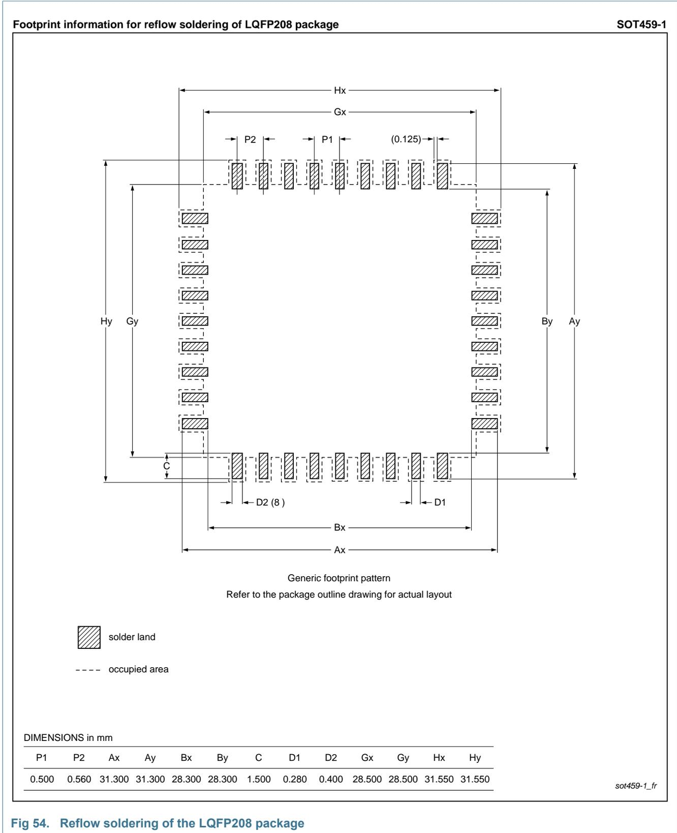
Fig 54. Reflow soldering of the LQFP208 package
