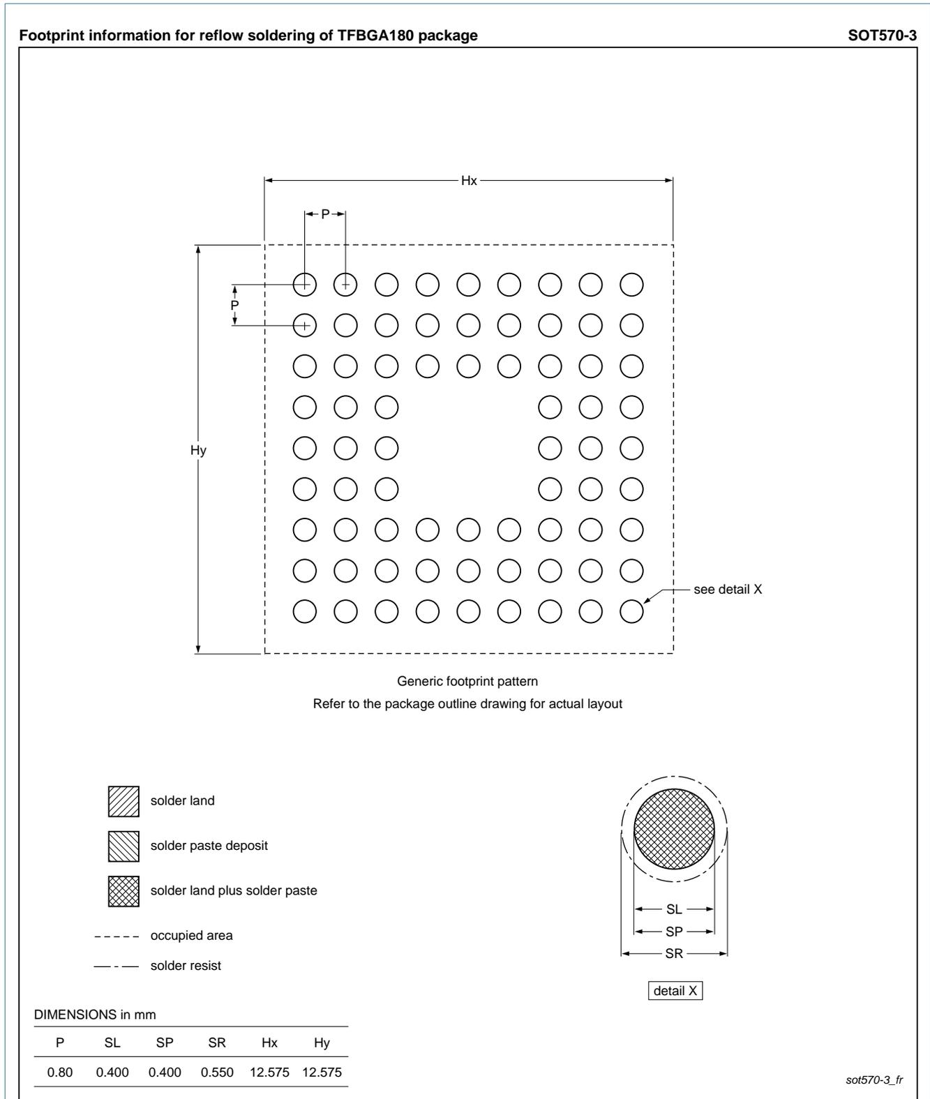
**Fig 56. Reflow soldering of the TFBGA180 package**
