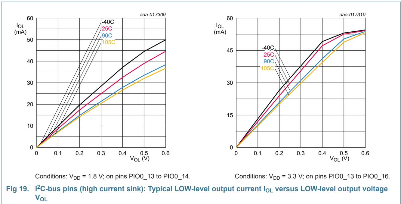
Fig 19. I<sup>2</sup>C-bus pins (high current sink): Typical LOW-level output current  $I_{OL}$  versus LOW-level output voltage  $V_{OL}$
