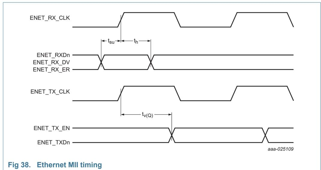
**Fig 38. Ethernet MII timing**
