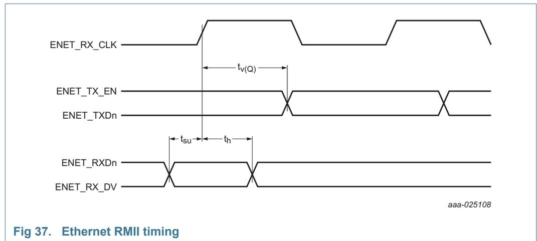
**Fig 37. Ethernet RMI timing**
