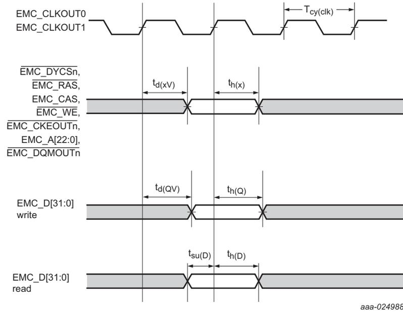
Fig 27. Dynamic external memory interface signal timing
