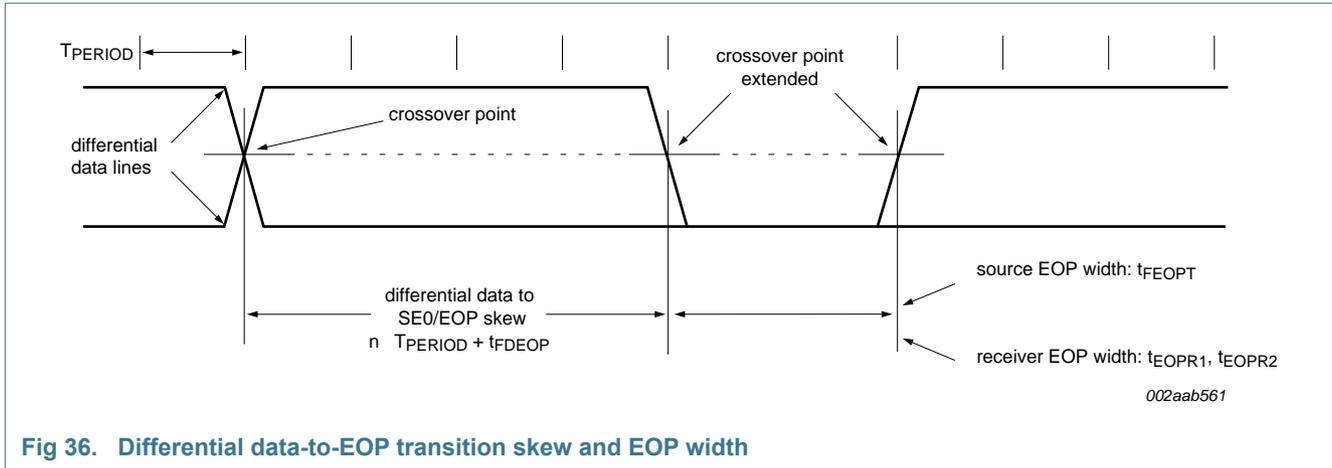
Fig 36. Differential data-to-EOP transition skew and EOP width
