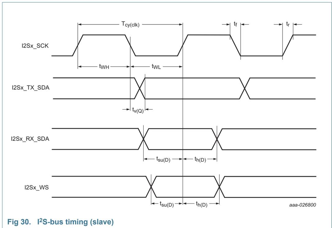
Fig 30. I<sup>2</sup>S-bus timing (slave)
