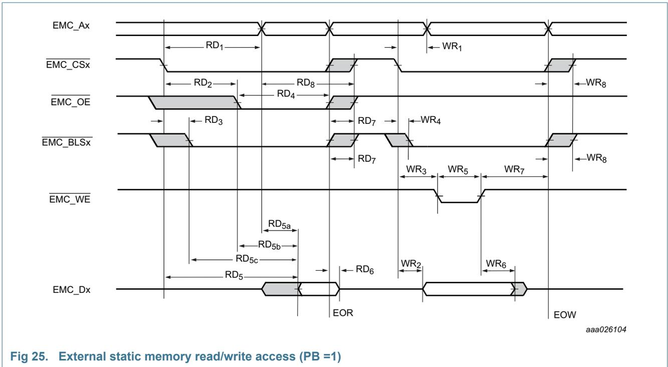
Fig 25. External static memory read/write access (PB = 1)
