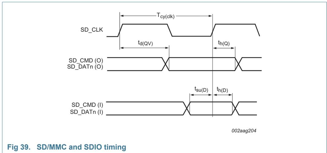
Fig 39. SD/MMC and SDIO timing
