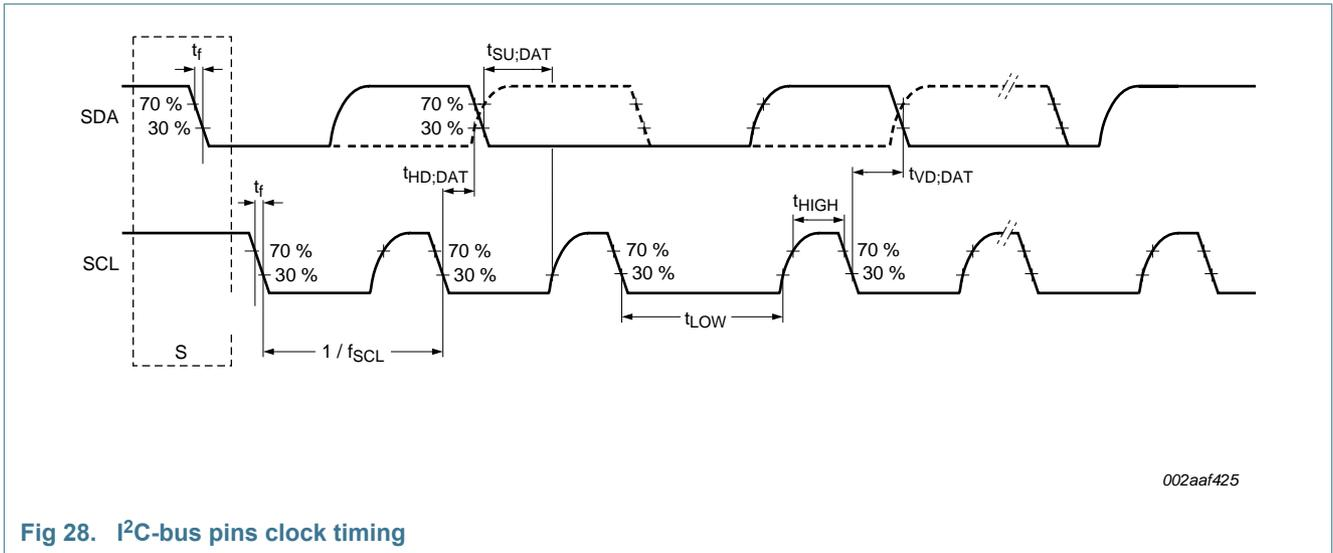
Fig 28. I<sup>2</sup>C-bus pins clock timing
