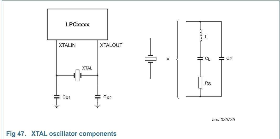
Fig 47. XTAL oscillator components
