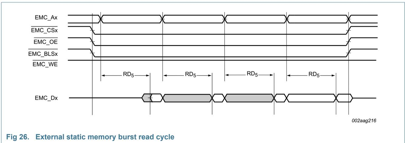
Fig 26. External static memory burst read cycle
