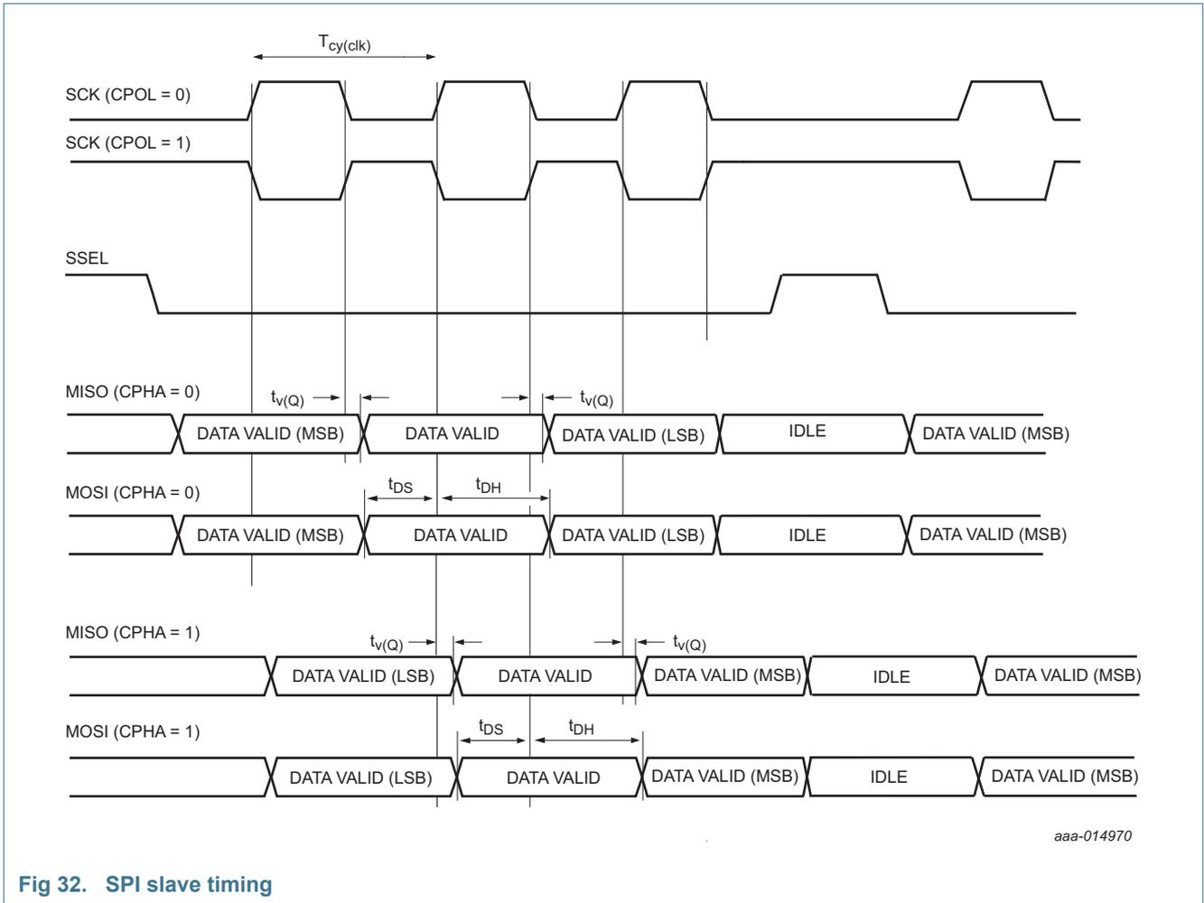
Fig 32. SPI slave timing
