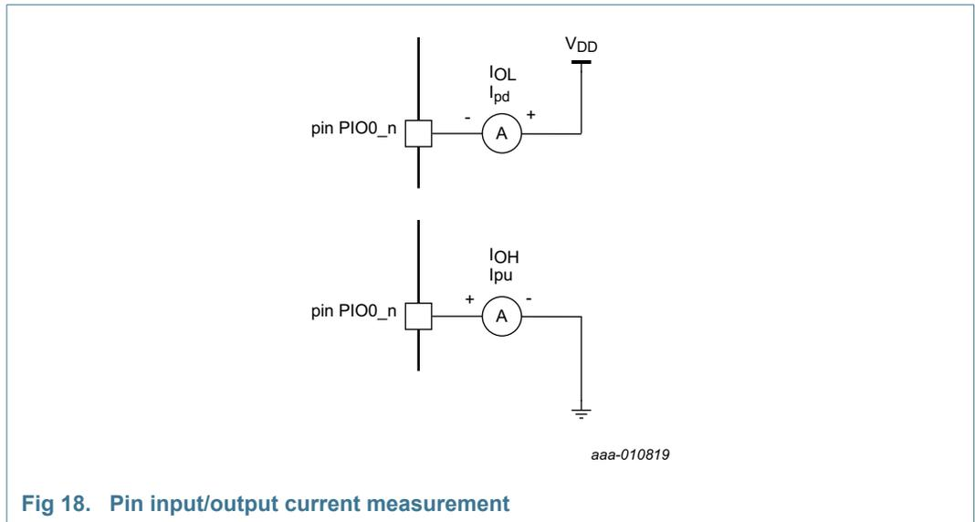
Fig 18. Pin input/output current measurement
