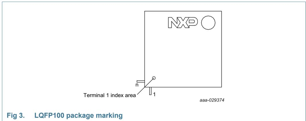
Fig 3. LQFP100 package marking
