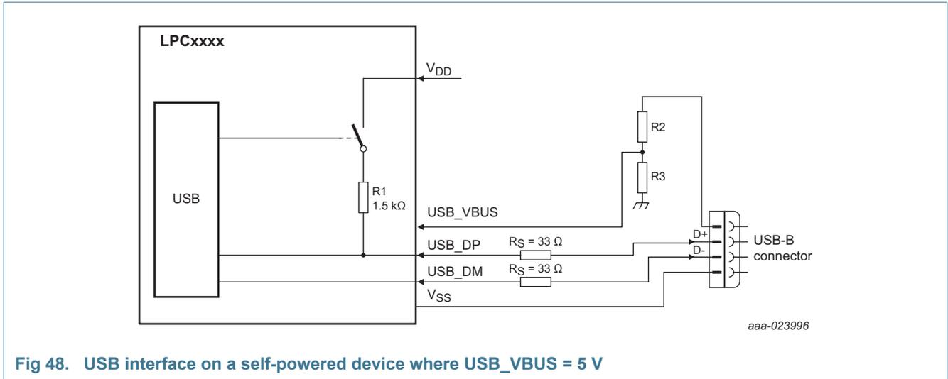
**Fig 48. USB interface on a self-powered device where USB\_VBUS = 5 V**
