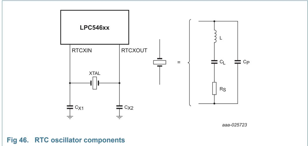
**Fig 46. RTC oscillator components**
