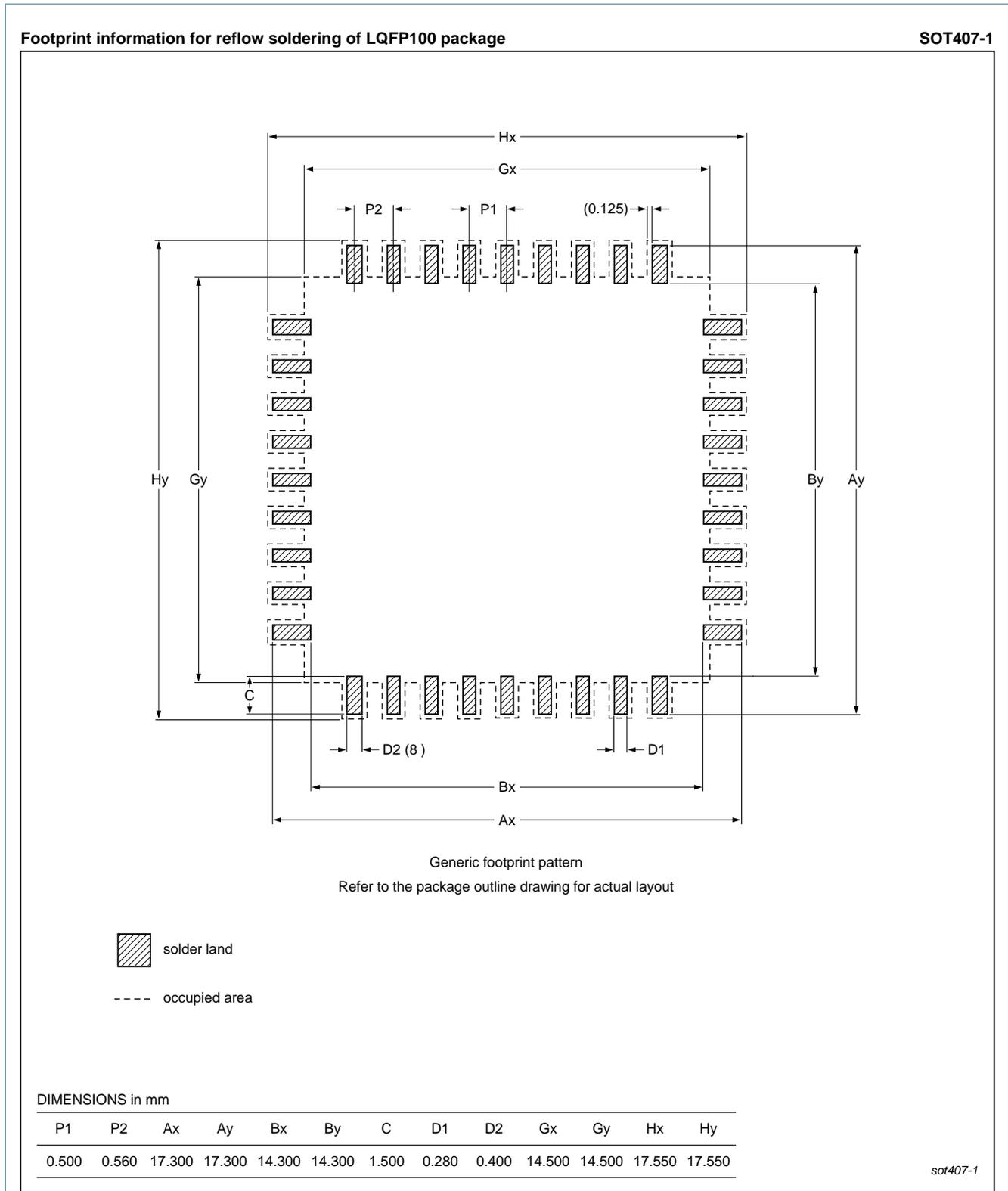
**Fig 55. Reflow soldering of the LQFP100 package**
