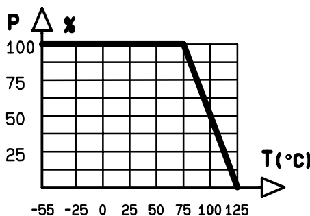
Power derating Versus temperature
