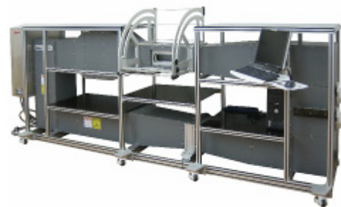
Fig. D: FDK Original Wind Tunnel
