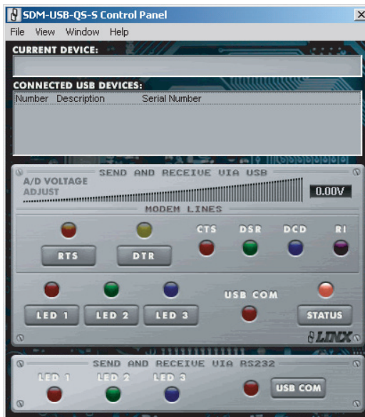
Figure 12: The Control Panel for RS-232 Operation
