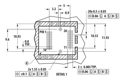
Figure 7. SFP Host Board Mechanical Layout
