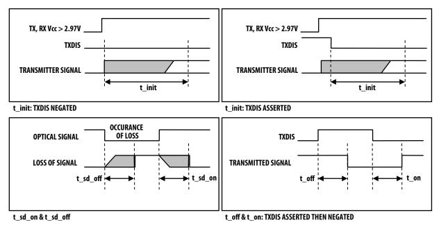
Figure 5. Timing diagrams
