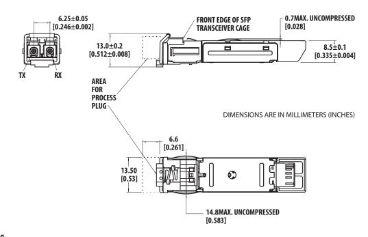
Figure 6. Module Drawing
