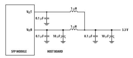
Note: Inductors must have less than 1 ohm series resistance per MSA.
