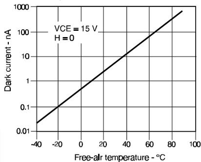
Fig. 4 Collector Current vs Ambient Temperature
