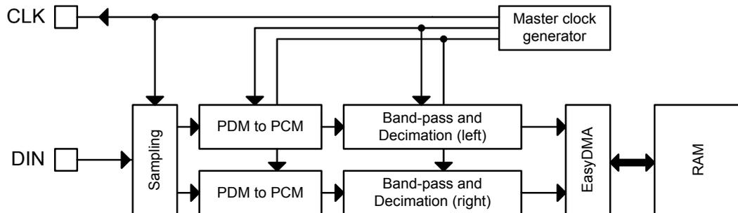
**Figure 123: PDM module**
