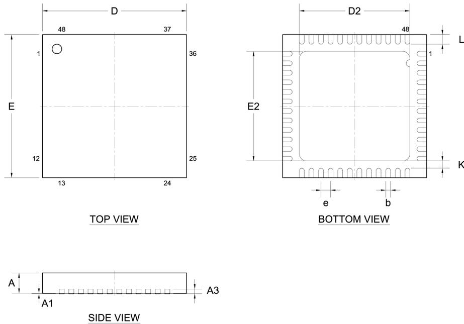
Figure 162: QFN48 6 x 6 mm package
