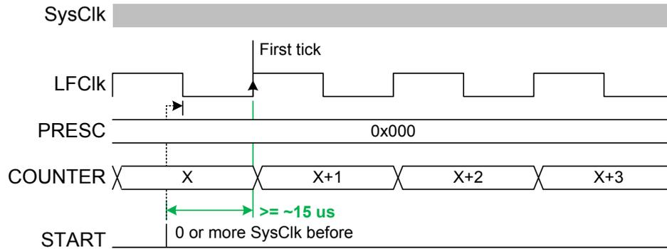
**Figure 54: Timing diagram - JITTER\_START-**
