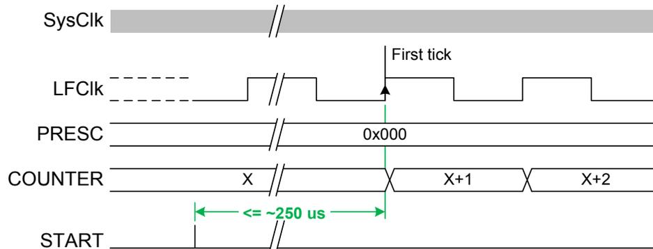
**Figure 55: Timing diagram - JITTER\_START+**
