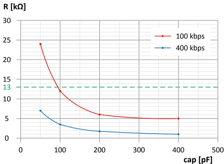
Figure 84: Recommended TWIM pullup value vs. line capacitance
