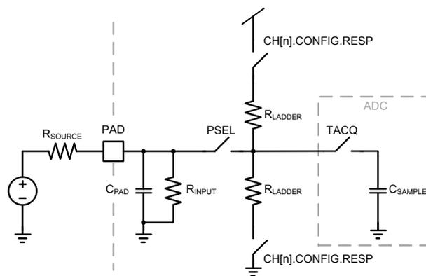
**Figure 104: Model of SAADC input (one channel)**
