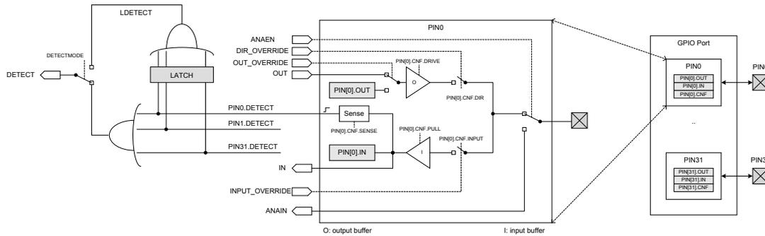
**Figure 20: GPIO Port and the GPIO pin details**
