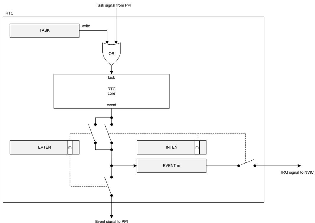
**Figure 45: Tasks, events and interrupts in the RTC**
