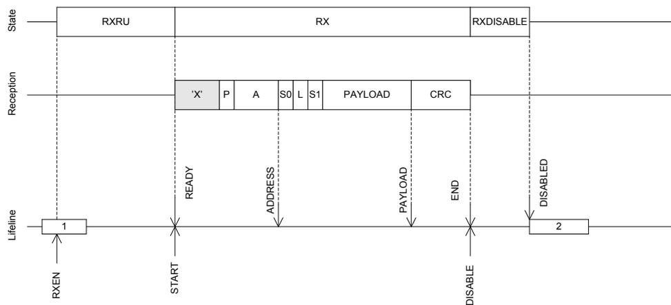
**Figure 38: Receive sequence using shortcuts to avoid delays**
