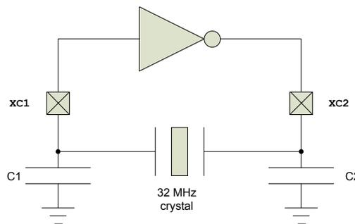
**Figure 17: Circuit diagram of the 64 MHz crystal oscillator**
