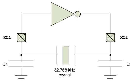
**Figure 19: Circuit diagram of the 32.768 kHz crystal oscillator**
