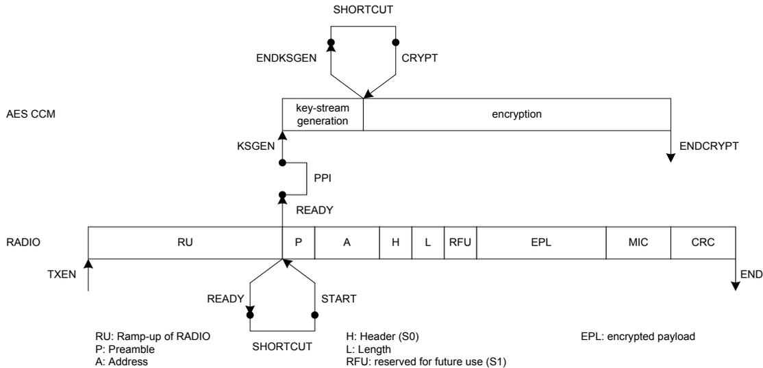
**Figure 62: On-the-fly encryption using a PPI connection**
