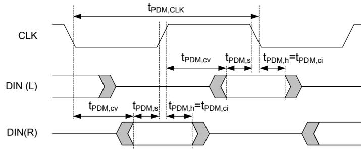
**Figure 127: PDM timing diagram**
