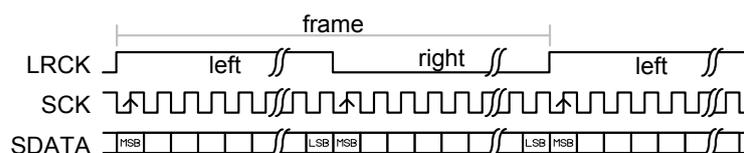
**Figure 132: Aligned format. CONFIG.SWIDTH equalling half-frame size.**
