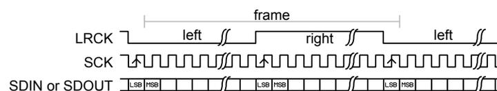
**Figure 131: I<sup>2</sup>S format. CONFIG.SWIDTH equalling half-frame size.**
