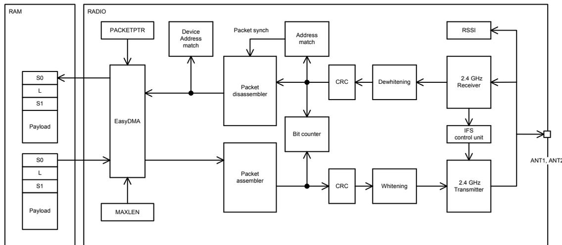
**Figure 28: RADIO block diagram**
