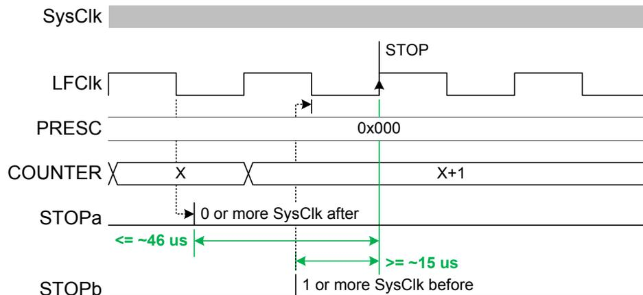
**Figure 53: Timing diagram - DELAY\_STOP**
