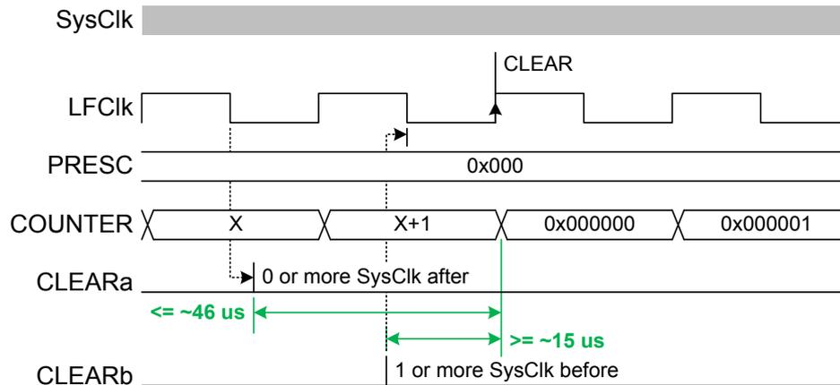
**Figure 52: Timing diagram - DELAY\_CLEAR**
