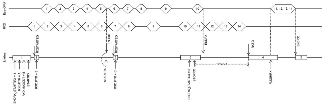
**Figure 95: UARTE reception with forced stop via STOPRX**
