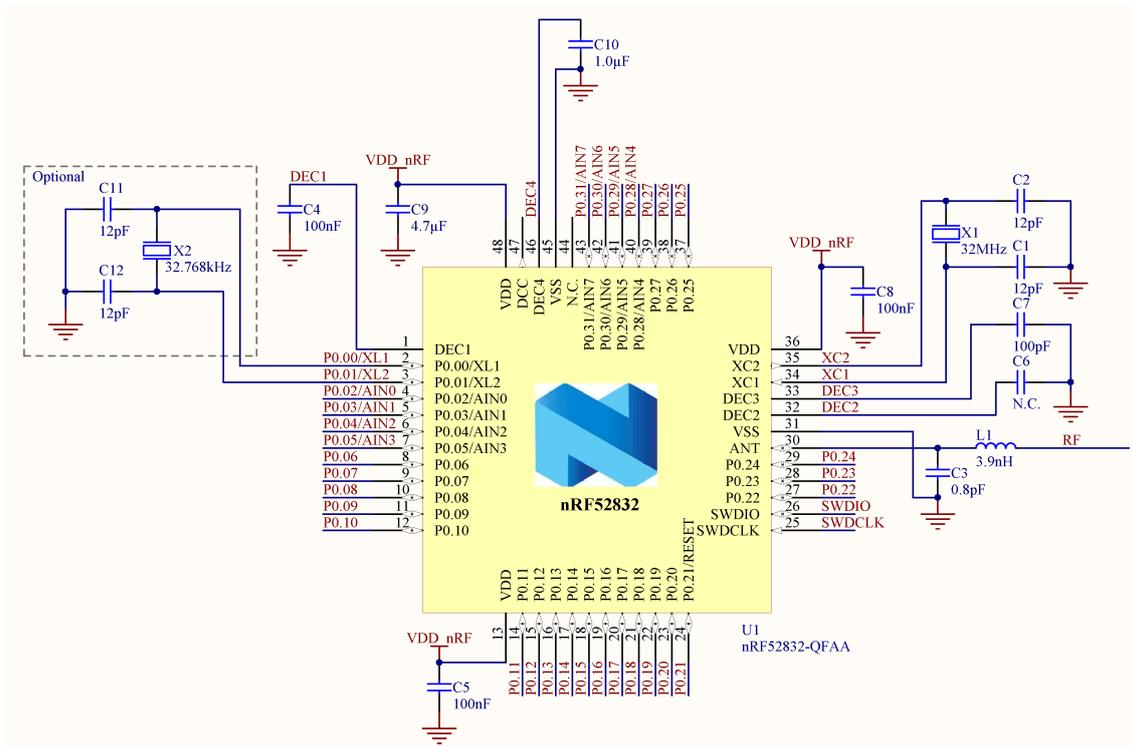
Figure 167: QFAA QFN48 with internal LDO setup
