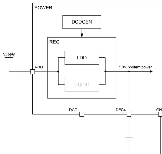
**Figure 12: LDO regulator setup**
