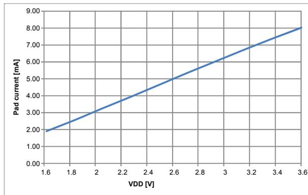
**Figure 24: Max sink current vs Voltage, standard drive**
