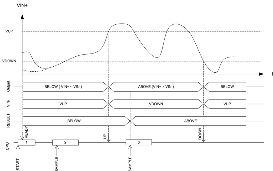
**Figure 112: Hysteresis example where VIN+ starts below VUP**
