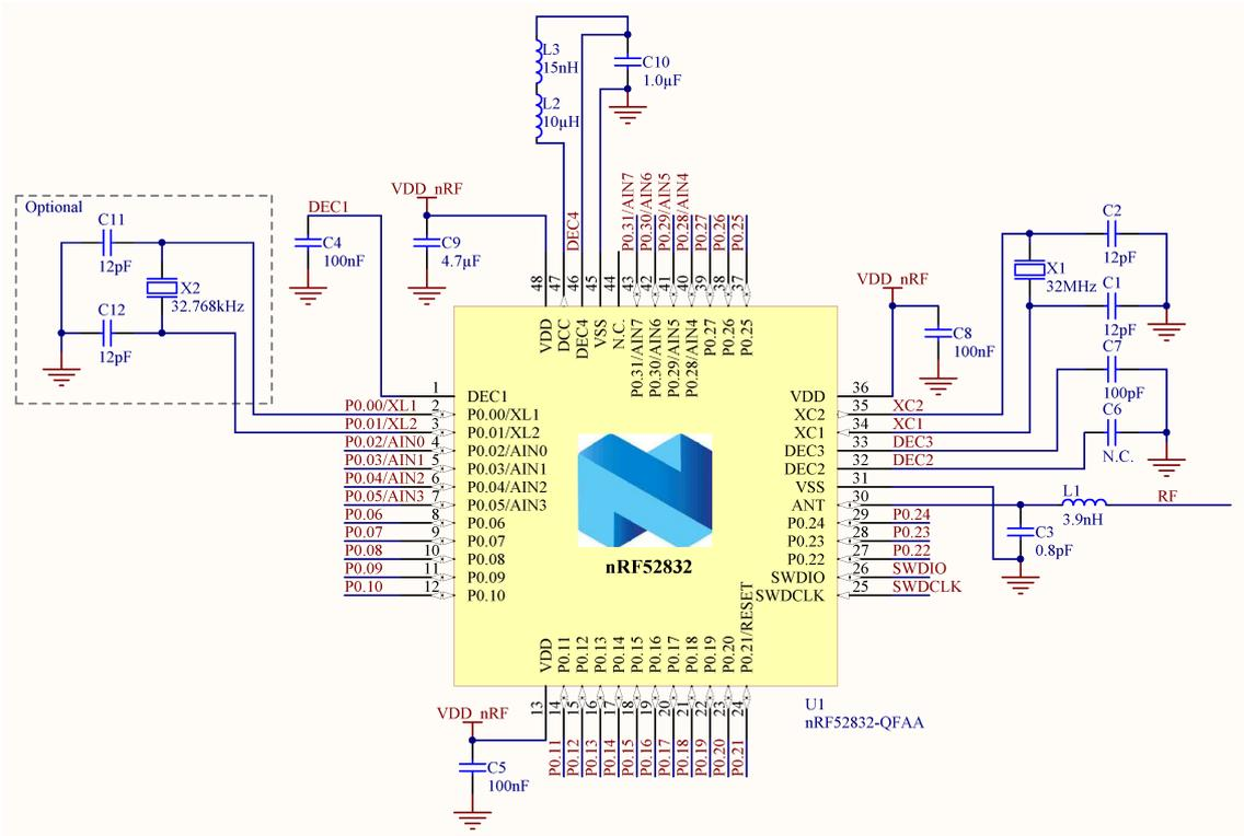
Figure 168: QFAA QFN48 with DC/DC regulator setup
