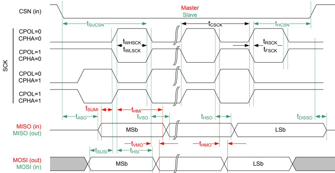
Figure 75: Common SPIM and SPIS timing diagram
