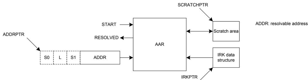
Figure 66: Address resolution with packet preloaded into RAM
