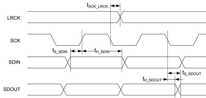
Figure 139: I2S timing diagram
