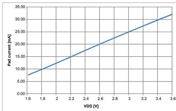
**Figure 25: Max sink current vs Voltage, high drive**
