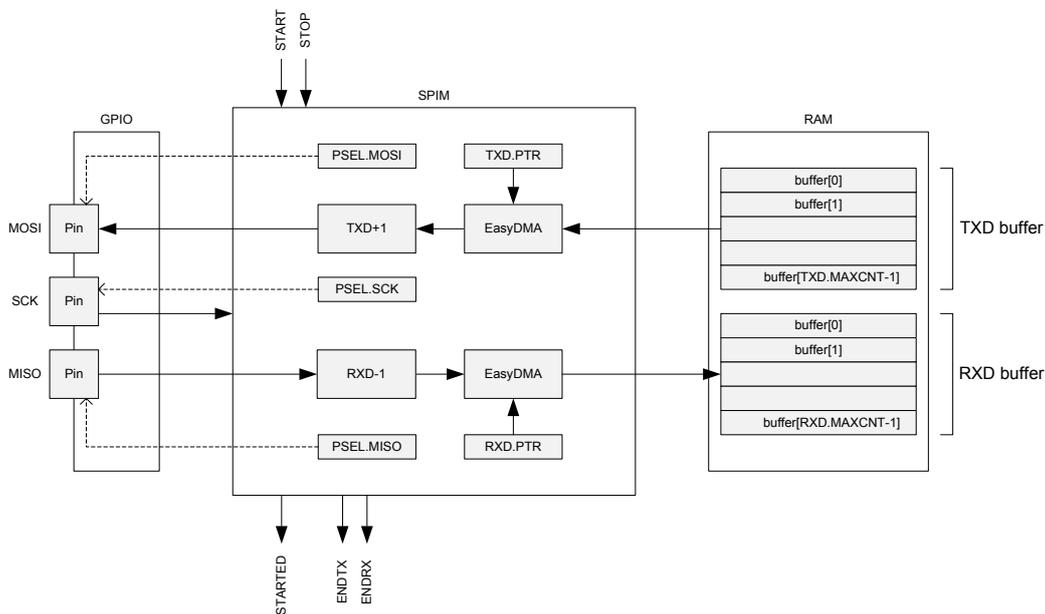
**Figure 68: SPIM — SPI master with EasyDMA**
