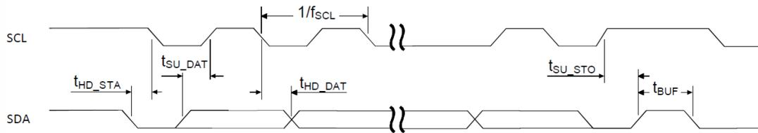
Figure 158: TWI timing diagram, 1 byte transaction
