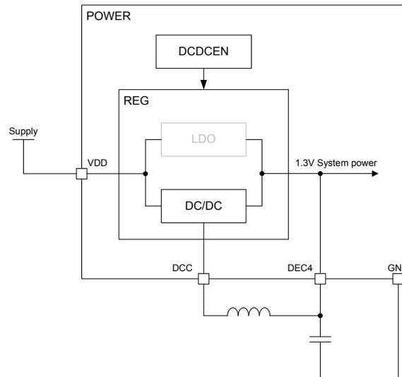
**Figure 13: DC/DC regulator setup**
