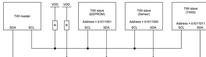
**Figure 86: A typical TWI setup comprising one master and three slaves**
