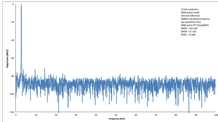
Figure 107: FFT of a 2.8 kHz sine at 200 ksps ()
