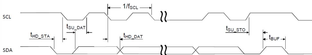
Figure 83: TWIM timing diagram, 1 byte transaction
