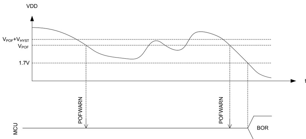
**Figure 15: Power-fail comparator (BOR = Brownout reset)**
