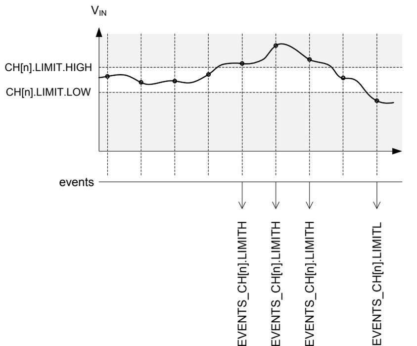
Figure 103: Example of limits monitoring on channel 'n'
