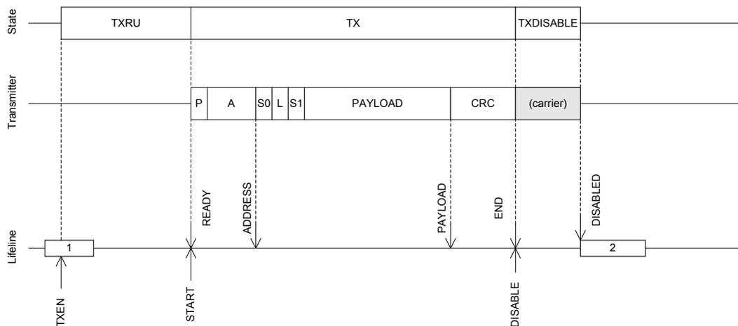
**Figure 35: Transmit sequence using shortcuts to avoid delays**
