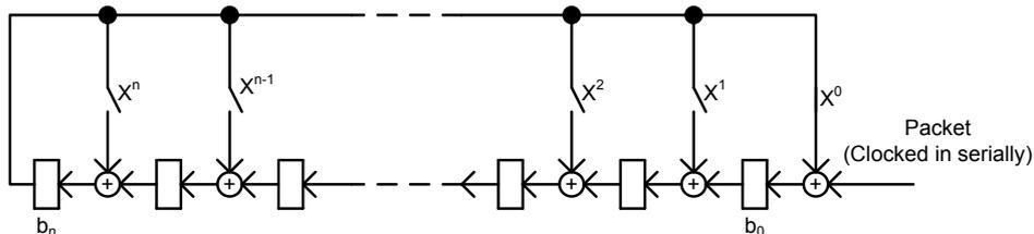
**Figure 32: CRC generation of an n bit CRC**
