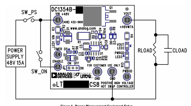
Figure 1. Proper Measurement Equipment Setup
