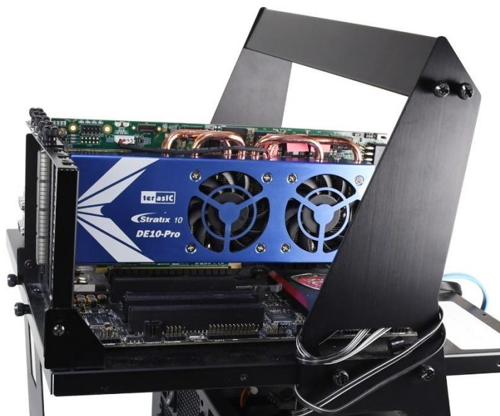
Figure 7-9 FPGA board installation on PC
