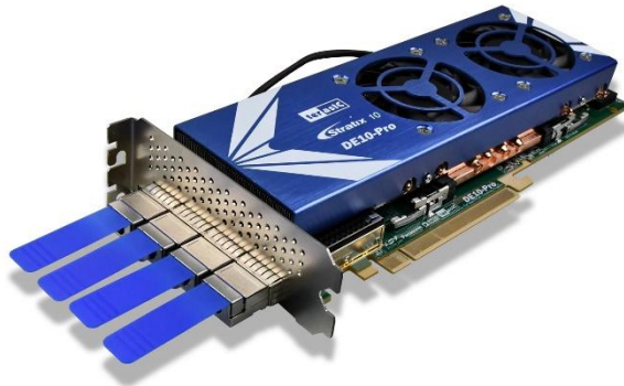
Figure 9-2 QSFP28 Transceiver Loopback Test in Progress
