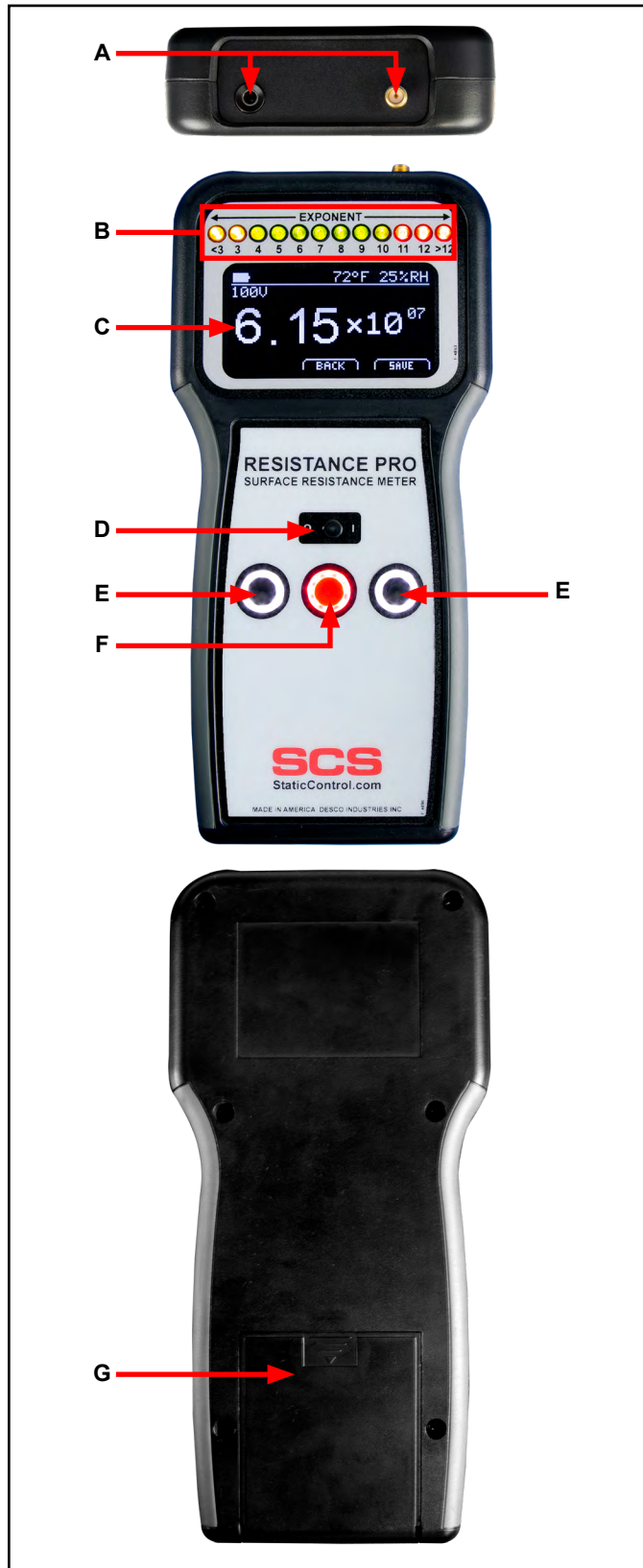
Figure 4. Resistance Pro Meter features and components
