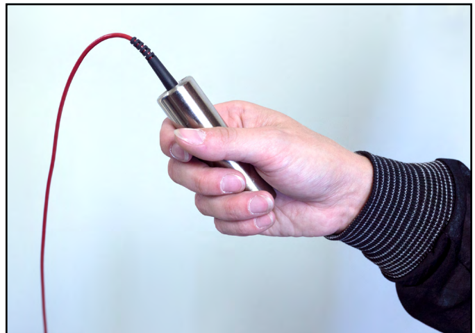
Figure 11. Using the SCS 770765 Handheld Electrode
