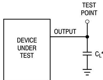
\*Includes all probe and jig capacitance
