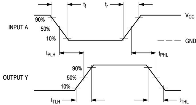
Figure 1. Switching Waveforms
