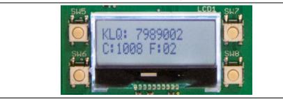
When a Classic KEELOQ packet is received from a paired transmitter, the contents of the packet is displayed on the LCD, as shown in Figure 2-6. Table 2-3 describes the data displayed on the screen.
