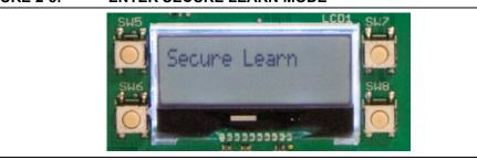
The receiver must complete the learn process within a fixed window. If the necessary data is not received from the transmitters within this window, the process will abort and a message similar to Figure 2-9 is displayed.
