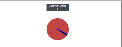
If the difference between a received synchronization counter and the last stored counter is within 16, the intended function will be executed on the single button press and the new synchronization counter will be stored. Storing the new synchronization counter value effectively rotates the entire Synchronization window.
