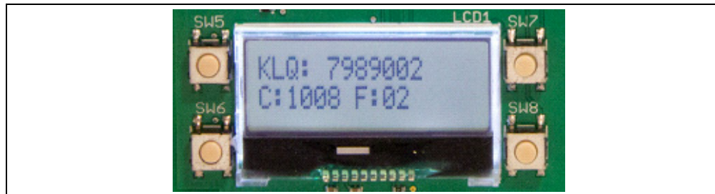
FIGURE 2-5: TYPICAL CLASSIC KEELOQ® TRANSMISSION
