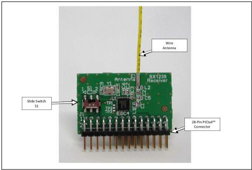
The daughter board features the Semtech SX1239 Low-Power Integrated UHF Receiver (http://www.semtech.com/wireless-rf/rf-receivers/sx1239/). The PICtail daughter board can plug into the 28-pin PICtail connector, featured on many Microchip Technology development tools.
