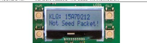
The synchronization counter is used to validate Classic Keelog transmissions. If the transmitted value falls outside the acceptable boundaries of the receiver's copy, an error similar to Figure 2-14 is displayed.
