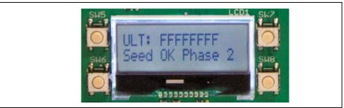
Ultimate KEELOQ requires an explicit transmission of a Typical packet. Once received, a message similar to the one shown in Figure 2-12 is displayed.
