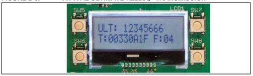
The kit can pair transmitters using Normal Learn or Secure Learn (note, though, that the included transmitters are configured to pair only using Secure Learn). When the receiver enters Normal Learn mode, text similar to Figure 2-7 is displayed. For Secure Learn, text similar to Figure 2-8 is shown.
