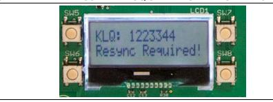
Packets from Ultimate Keelog encoders are always validated initially by confirming the Authorization Code portion of the transmission. If this check fails, a message similar to Figure 2-15 is displayed. Note that, this may be seen while completing the Secure Learn process and does not necessarily indicate an error.
