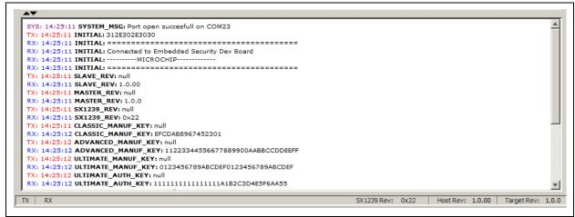
Notice how the toolbar lists the software revisions of the Host and Target microcontrollers. The GUI will only communicate with known revisions of the firmware. The SX1239 is the identification number of the SemTech receiver module. Please see the SemTech data sheet for much more information regarding their receiver. Other settings such as learned devices and manufacturing numbers are also displayed and saved.
