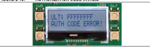
The kit allows the user to erase, or 'forget', all paired transmitters. If done, the LCD will display a message similar to Figure 2-16.
