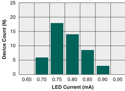
Typical I<sub>F</sub> for Switch Dropout
