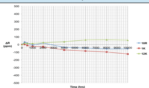
FIGURE 6 - LOAD LIFE TEST FOR 10,000 HRS @0.3W, +70°C; VSMP 1206, N=40
