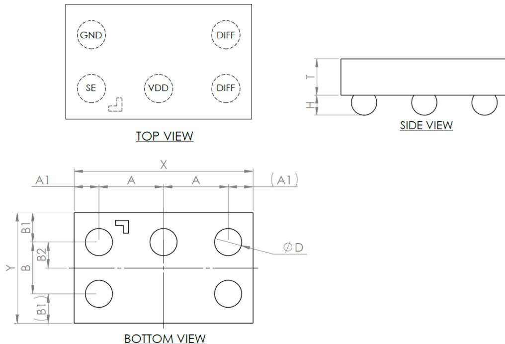
Table 4. Ultra thin Flip-Chip 5 bumps package mechanical data
