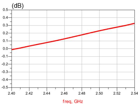
**Figure 6. Phase imbalance ( $T_{amb} = 25^{\circ}\text{C}$ )**
