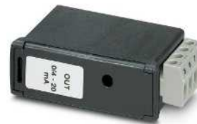
Two analog outputs
