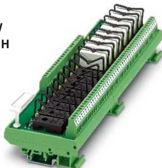
16-channel for relays with a PDT contact
