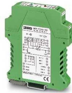
For Pt 100, either voltage or current output
