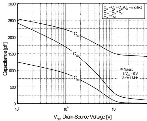
Figure 5. Capacitance Characteristics
