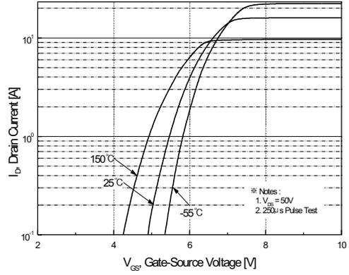
Figure 2. Transfer Characteristics
