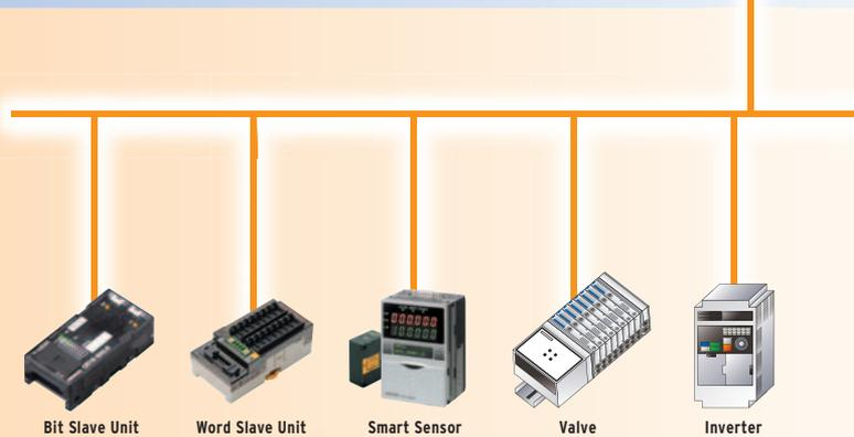
"CompoNet" globally standardized open network in the sensor & actuator layer
