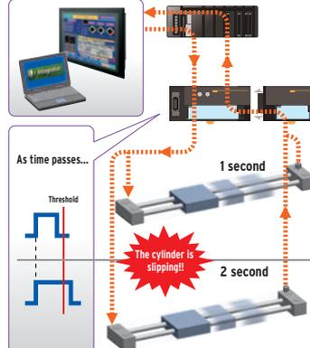
The slave unit counts the machine's ON/OFF repetitions and total operation time to let you know when it is time for maintenance. (Contact operation monitor)
