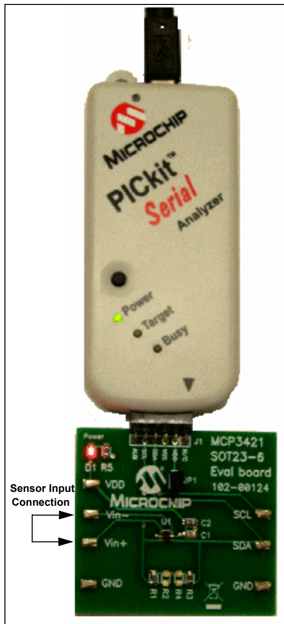
FIGURE 7-2: Setup for the MCP3421 Evaluation Board with PICKit™ Serial Analyzer.
