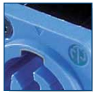
Locking area on chassis connector
