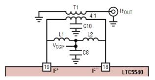
Figure 1. IF Output with Bandpass Matching
