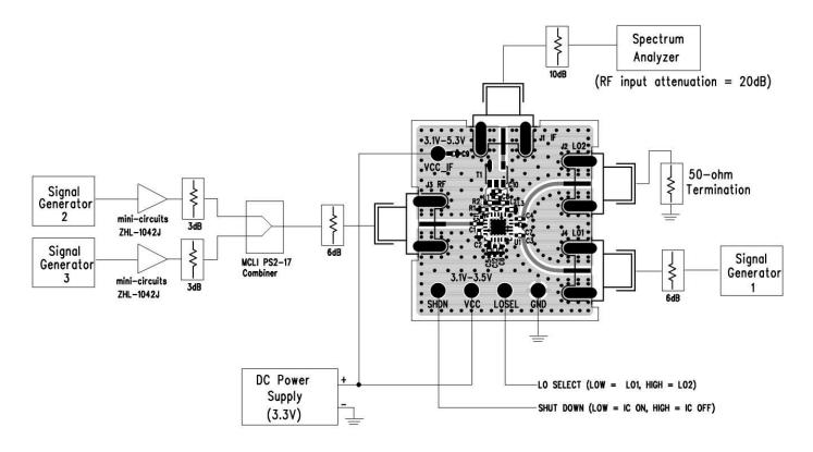
Figure 6. Proper Equipment Setup for RF Performance Measurements
