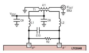
Figure 3. IF Output with Lowpass Matching
