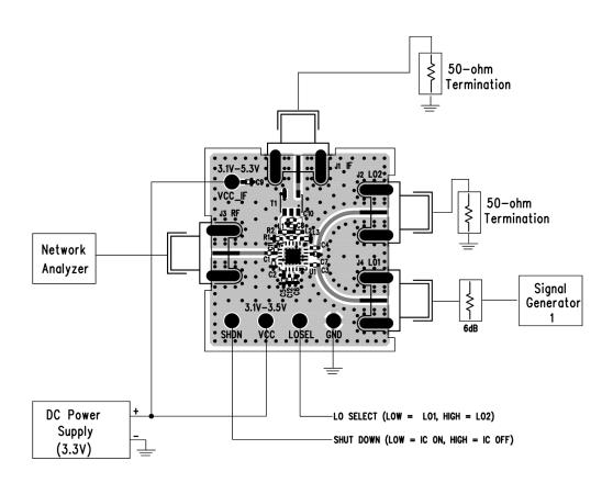
Figure 5. Proper Equipment Setup for Return Loss Measurements
