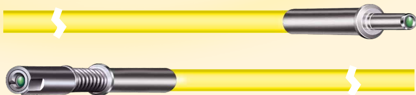
Factory terminated lens pin contact (top) and lens socket contacts on pigtail wires allow for easier fusion splicing in the field.
