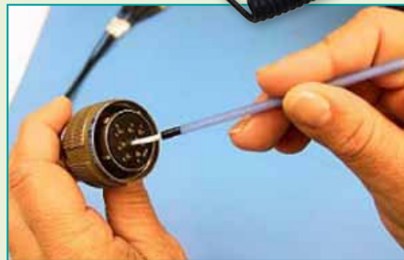
Compressed-air cleaning of a connector face, and swab cleaning of ferrule/fiber end of socket termini
