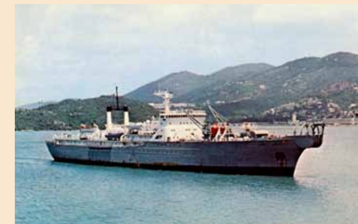
CS Long Lines, a ship designed to lay the Trans-Atlantic fiber optic cable for AT&T. This ship was used to conduct the first deep-sea trials of fiber optic cable in 1982. AT&T laid and opened the first fiber-optic cable across the Atlantic in 1988.
