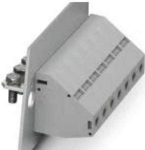
Panel feed-through terminal block, Connection method: Screw connection, Screw connection, Load current : 150 A, Cross section: 16 mm 2 - 50 mm 2 , AWG 6 - 1/0, Width: 18.8 mm, Color: gray
