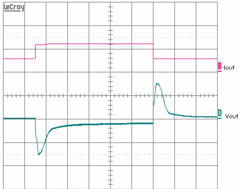
Figure 5. Transient Response Waveform at 48Vin and 5 - 6Aout – 200μS, 5A, and 200mV / div
