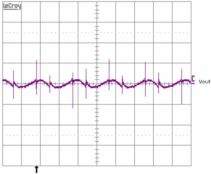
Figure 4. Output Ripple at 48Vin and 6Aout (20MHz) - 2μS and 20mV / div
