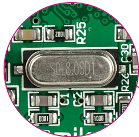
Figure 5-1: External crystal oscillator (X1)
