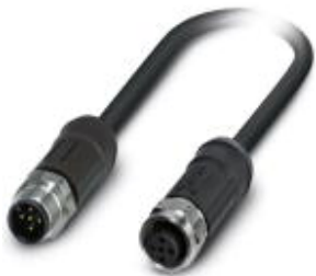
Sensor/Actuator cable, 5-position, PE-X halogen-free, black-gray RAL 7021, Plug straight M12, A-coded, on Socket straight M12, A-coded, Cable length: 2 m, for outdoor applications, with high-grade steel knurl
