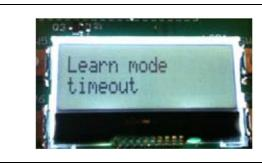
When all slots in the NVM space for transmitters are taken, the learning process fail. Press and hold **SW4** button for about ten seconds to erase all transmitter records from the NVM. The message "Memory Erased" displays on the LCD as shown in Figure 2-6. After erasing records from the NVM, reset the board by removing and reinserting J6.
