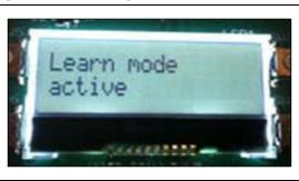
If the received packet is from a known transmitter, the NVM remains untouched. If a relearn is performed to resynchronize the hop counter of a transmitter, the NVM must be erased first. If no Keelog Classic packet from an unknown transmitter is received within 18 seconds, the Keelog Classic Learn mode timeouts and displays the message "Learn mode timeout" on the LCD as shown in Figure 2-5.
