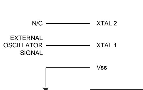
**Figure 2. External Clock Drive configuration**
