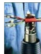
Applying Shrink Tubes
