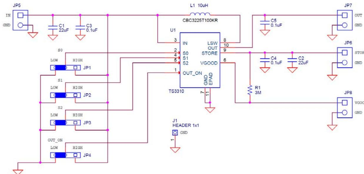
**Figure 2.1. TS331x-EVB Schematic**
