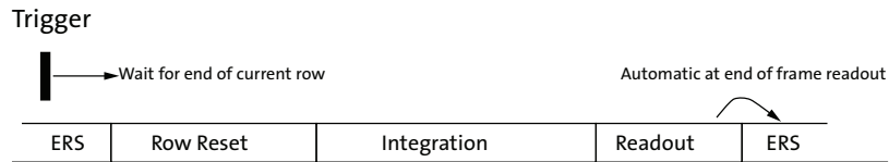
Figure 47: Entering and Leaving a Global Reset Sequence
