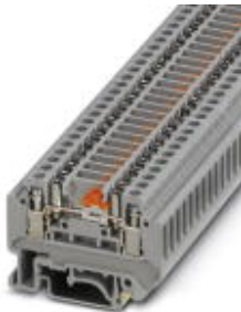
Disconnect terminal block, Connection method: Screw connection, Cross section: 0.2 mm 2 -4 mm 2 , AWG: 24 - 12, Width: 6.2 mm, Mounting type: NS 35/7,5, NS 35/15, NS 32, Color: gray
