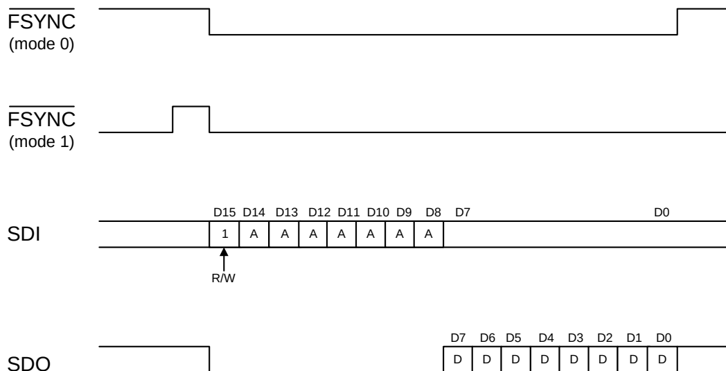
Figure 29. Secondary Communication Data Format—Read Cycle
