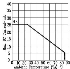
Fig5. MAX. ALLOWABLE DC CURRENT VS. AMBIENT TEMPERATURE.
