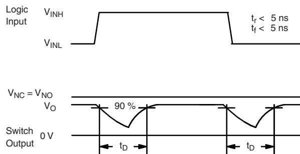
Figure 2. Break-Before-Make Interval
