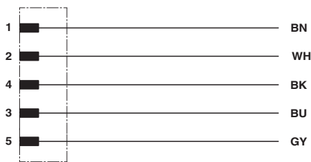
Contact assignment of the M12 plug
