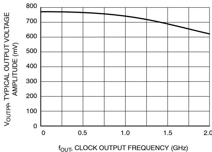
**Figure 22. Output Voltage Amplitude ( $V_{OUTPP}$ ) vs.
