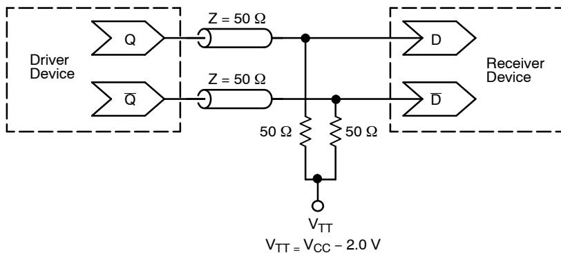
**Figure 21. Typical Termination for Output Driver and Device Evaluation
