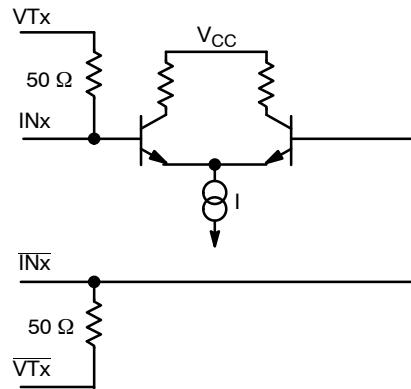
**Figure 9. Input Structure**
