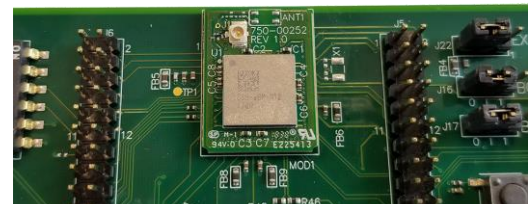
Figure 1: 455-00030 Sterling-EWB Development Kit w/ Chip Antenna
