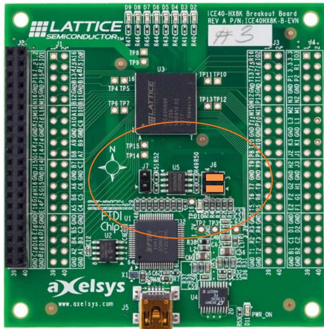
LED in location D10 is connected to the CDONE pin of the iCE40HX-8K. This can be monitored to determine that the iCE40HX-8K is programmed correctly.
