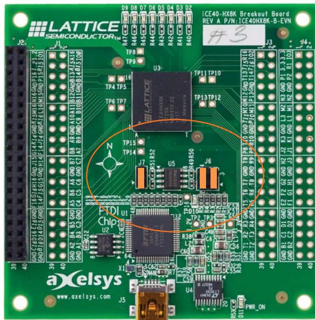
In SPI Peripheral Mode the SPI signals loads the program file into the CRAM (configuration ram) of the FPGA directly. In this mode the FPGA will lose its configuration when power is removed and must be re-configured. Jump-
