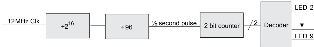
The source code has two counters that are used to divide the 12MHz clock by 216 and 96 generating an approximately  $\frac{1}{2}$  second pulse. This pulse along with the decoder will turn the LEDs (D2 thru D9) on for  $\frac{1}{2}$  second and off for  $\frac{1}{2}$  second. The decoder can be modified to have any type of LED sequence by changing either the VHDL or Verilog code.
