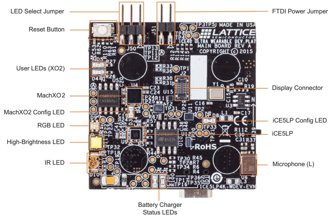
**Figure 2. Main Board (Bottom Side)**
