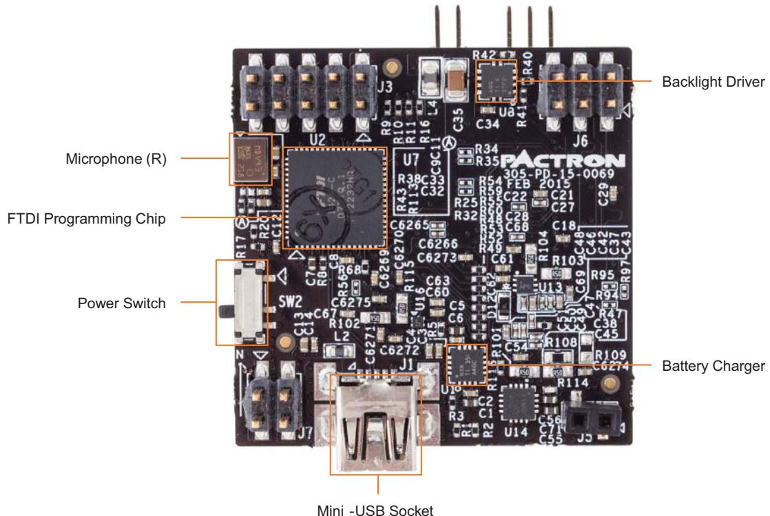
**Figure 3. Sensor Board (Top Side)**
