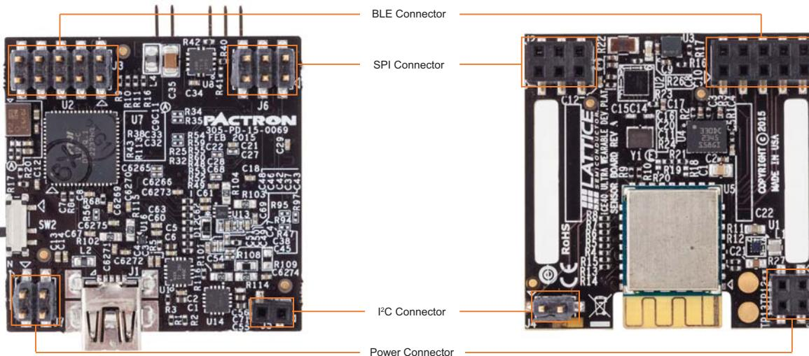
**Power Connector** (Main Board J7, Sensor Board J5): Power connection between the two boards
