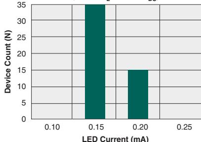
**Typical  $I_F$  for Switch Dropout
