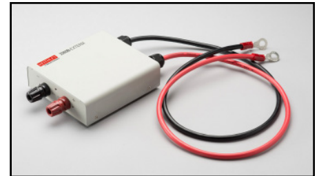
Model 2260B-EXTERM: Extended terminal; Test Leads, 0.7m (28 in.), and terminal box to bring outputs to the front of the instrument or another location. Magnetic base attaches to side of instrument.
